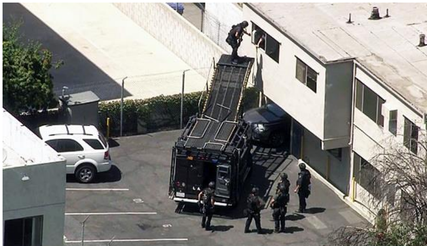
LAPD uses the Liberator ETS system during a Barricade situation to remove the suspect from his apartment.
