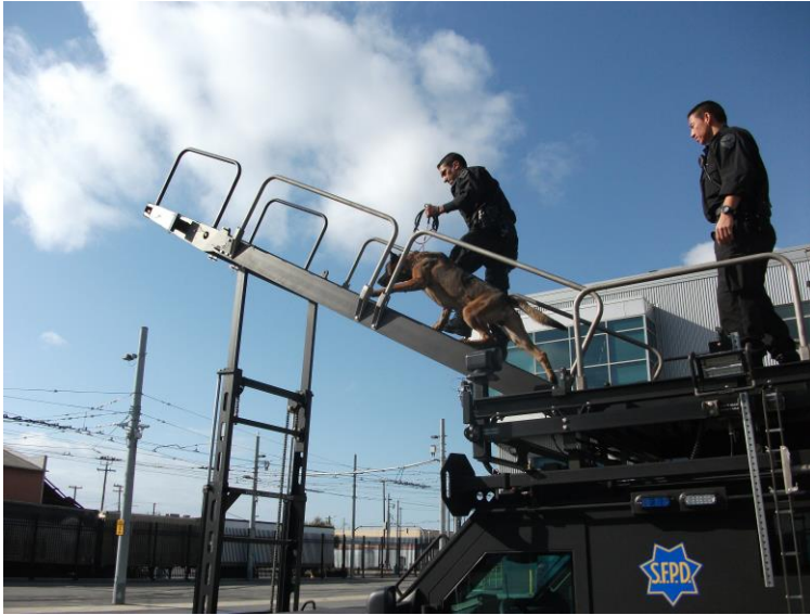
San Francisco Police practice using the Liberator to deploy K9s into elevated windows, balconies, doors.
