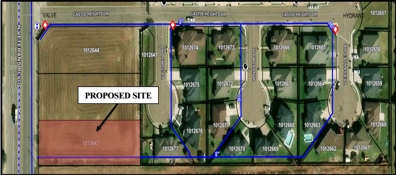
Water Map showing an 8-inch water line along 20-foot utility easement
